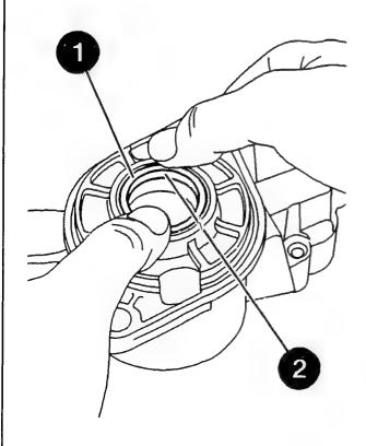
Checking drive-end bearing
